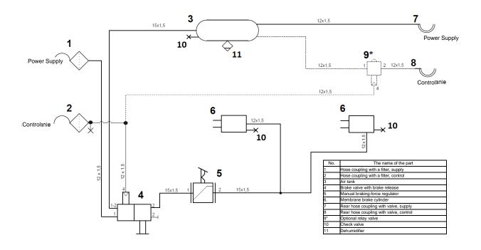
**Figure 15.** A diagram of a double-line pneumatic system - manual regulator without a relay (one cylinder per axle)
