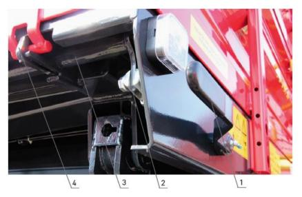
Figure 18. The locks on the sideboards of the load-carrying body (1-central lever of the bottom locks, 2-lock adjustment mechanism, 3-central lock shaft, 4-lock)
