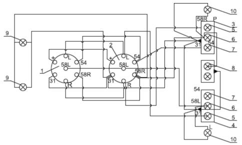
Figure 11. The trailer's wiring diagram (a version without side running lights)
