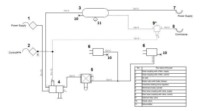
Figure 13. A diagram of a double-line pneumatic system - ALB, without a relay valve
