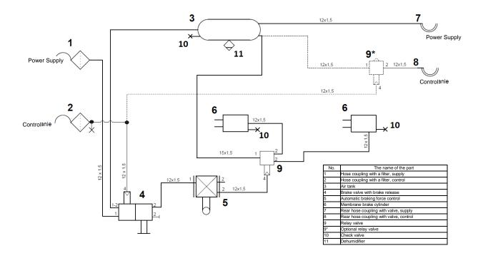
Figure 14. A diagram of a double-line pneumatic system - ALB, without a relay valve (one cylinder per axle)
