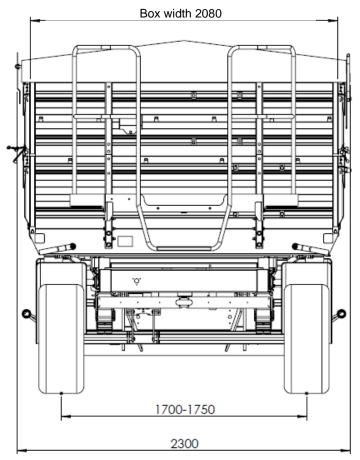
Figure 8. Dimensions of the trailer - front view
