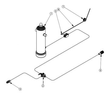
**Figure 10.** The diagram of the hydraulic system in the tilting mechanism of the trailer's body: 1 – cylinder, 2 – switching valve, 3 – cut-off valve, 4 – a plug of the connecting valve, 5 – connecting valve socket, 6 – control cable for the cut-off valve, 7 – cable roller
