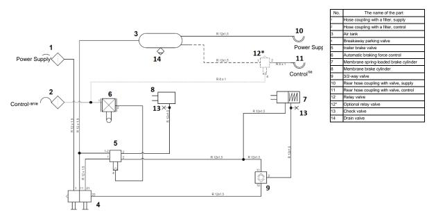
Figure 17. A diagram of the brake system with membrane spring-loaded cylinders and a relay valve
