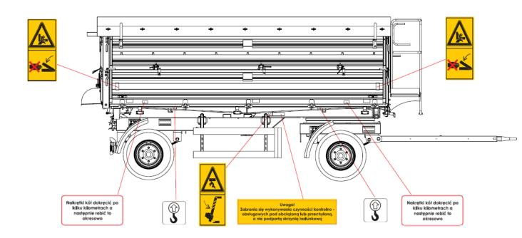
Figure 5. The arrangement of the pictograms on the boards of the trailer - right side
